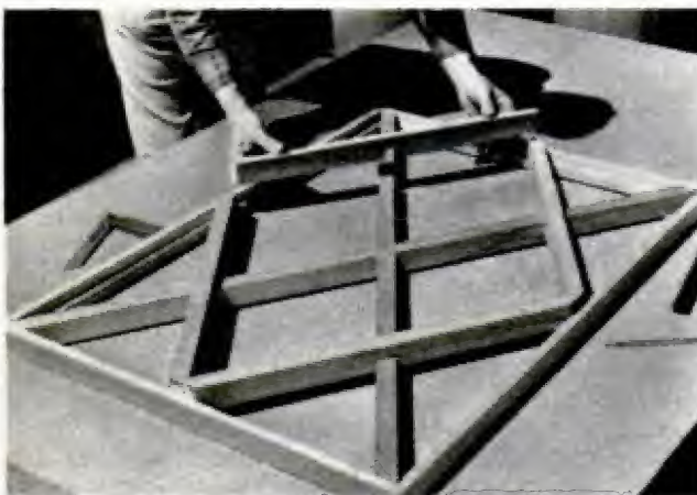
ROUTER AND SHAPED CUTTER dress up strips. Make sure that parts are numbered before disassembling
